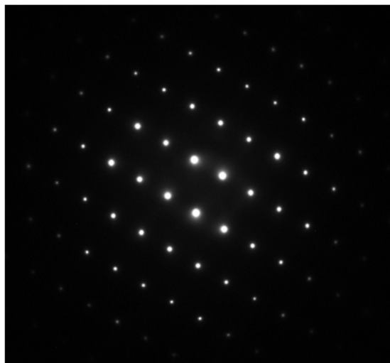
FIGURE 3.7: A typical electron diffraction pattern. This pattern is from an aluminum grain.
